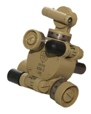
A sighting device NSB-3 is an optomechanical sight, that serves for taking firing elements on elevation and azimuth during direct, semi-indirect and indirect aiming from mortars up to 82mm caliber.
